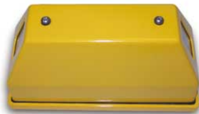
The propriety yellow casing on the outside of the bus discretely conceals the stop arm sentry.
